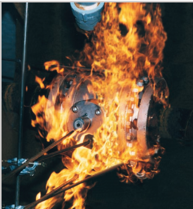
API-6FA firesafe test in process at Anderson & Associates in Houston, Texas.
